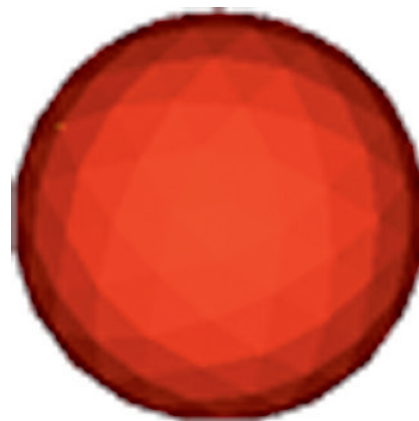
Fig. 1. Spherical grain embedded inside unit cube. The rate of interfacial area change can be analytically solved using the curvature driven growth relation. Following MacPherson–Srolovitz relation, the rate of volume change is dependant on the mean width since the structure lacks triple lines.
